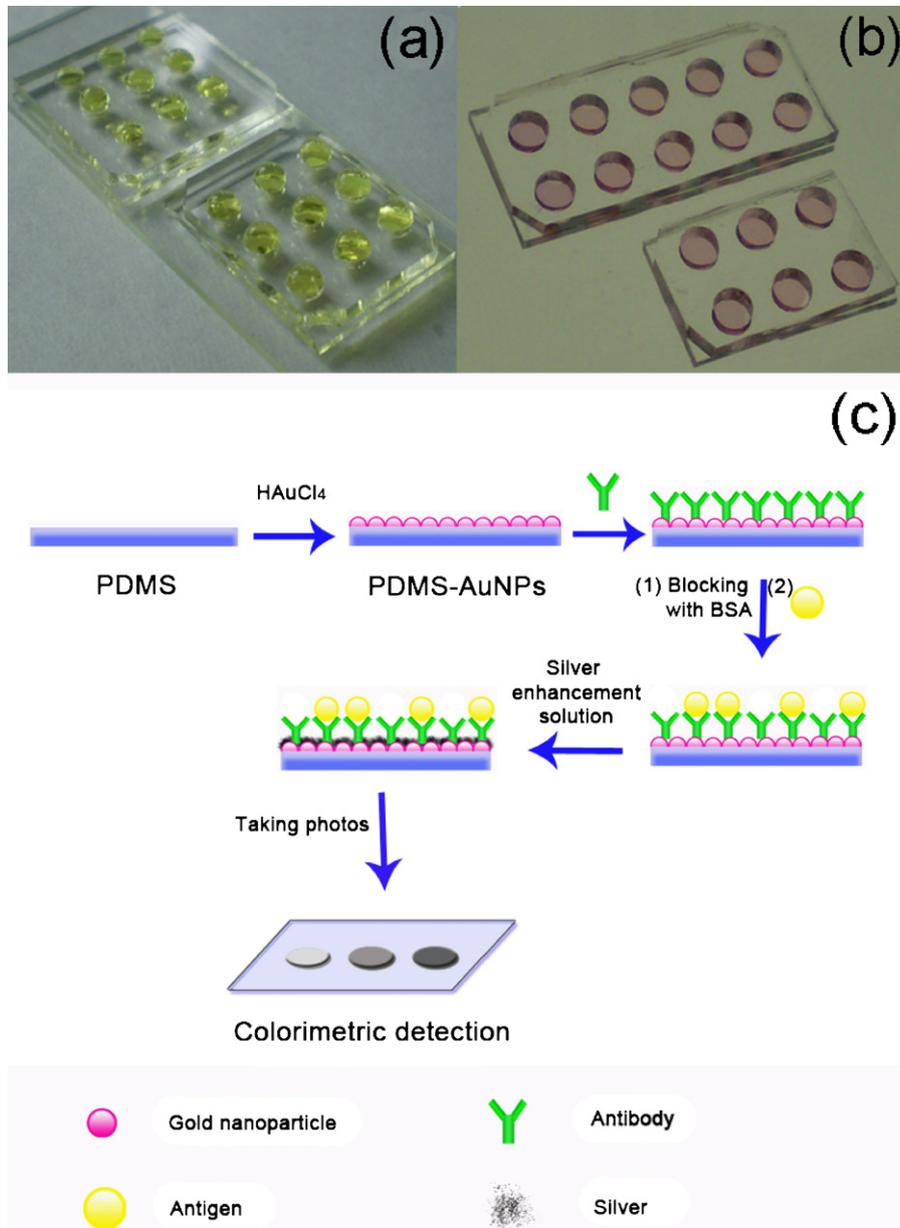
**Fig. 1.** Experimental procedure for silver enhancement colorimetric detection of cardiac troponin I; (a) is the PDMS chip with  $\text{HAuCl}_4$  solution; (b) is the photo of PDMS-AuNPs composite film; (c) schematic diagram for colorimetric detection.
