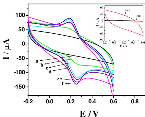
**Fig. 1** Cyclic voltammograms of different modified electrodes in pH 7.0 PBS containing 0.1 M KCl at a scan rate of  $50 \text{ mV s}^{-1}$ . *a* CILE, *b* HlgG/BSA–anti-HlgG/AuNPs/APS/PB/CILE, *c* BSA–anti-HlgG/AuNPs/APS/PB/CILE, *d* anti-HlgG/AuNPs/APS/PB/CILE, *e* APS/PB/CILE, and *f* AuNPs/APS/PB/CILE
