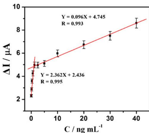
**Fig. 6** Calibration curve of the immunosensor for HIgG determination
