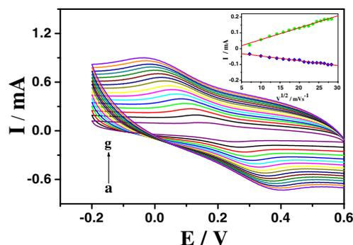
**Fig. 2** CVs of the immunosensor in pH 7.0 PBS containing 0.1 M KCl at different scan rates of (from inner to outer):  $50, 100, 150, 200, 250, 300, 350, 400, 450, 500, 550, 600, 650, 700, 750,$  and  $800 \text{ mV s}^{-1}$ . The inset shows the linear relationship between the peak currents and the square root of scan rate
