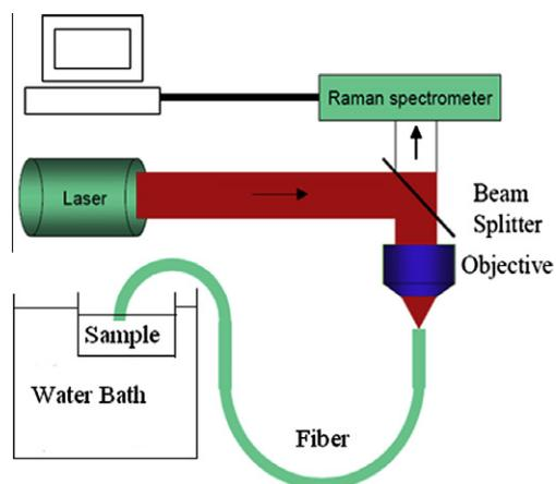
**Fig. 1.** Schematic of temperature-dependent SERS measurements using a single optical fiber.
