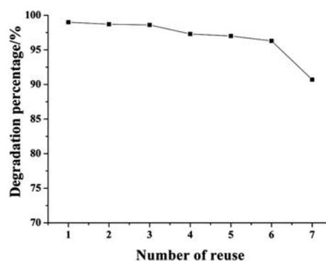
Fig. 13 Cycling runs in the photocatalytic degradation of MB in the presence of MoO<sub>3</sub> nanobelts under visible light irradiation.
