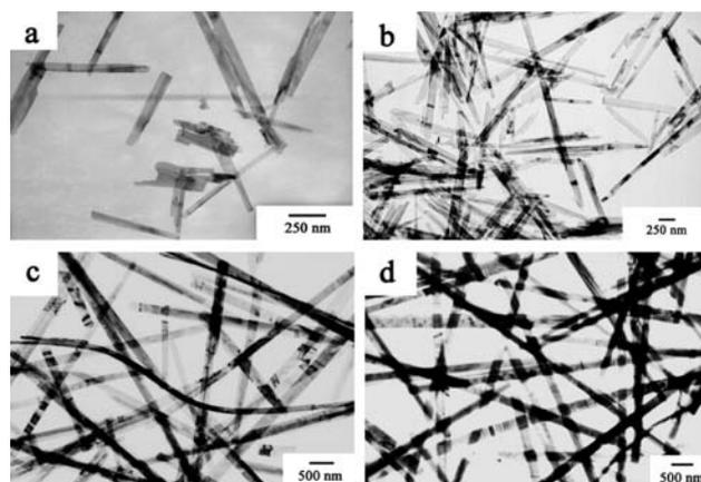
Fig. 10 TEM images of the products collected at different reaction time intervals in the presence of TX-10 (reaction temperature = 180 °C): (a) 5 min, (b) 0.5 h, (c) 5 h, (d) 20 h.
