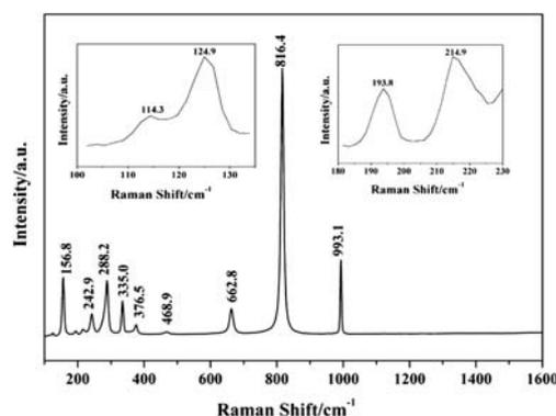
Fig. 7 Raman spectra of the as-synthesized MoO<sub>3</sub> nanobelts.
