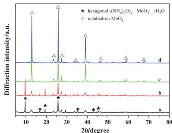
Fig. 8 XRD patterns of the as-prepared products obtained at different reaction time intervals in the presence of TX-10 (reaction temperature = 180 °C): (a) 5 min, (b) 0.5 h, (c) 5 h, (d) 20 h.
