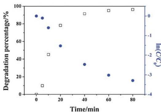
Fig. 12 Degradation percentage of MB (10 mg L<sup>-1</sup>, 100 mL) in the presence of MoO<sub>3</sub> nanobelts (50 mg) under visible light irradiation.
