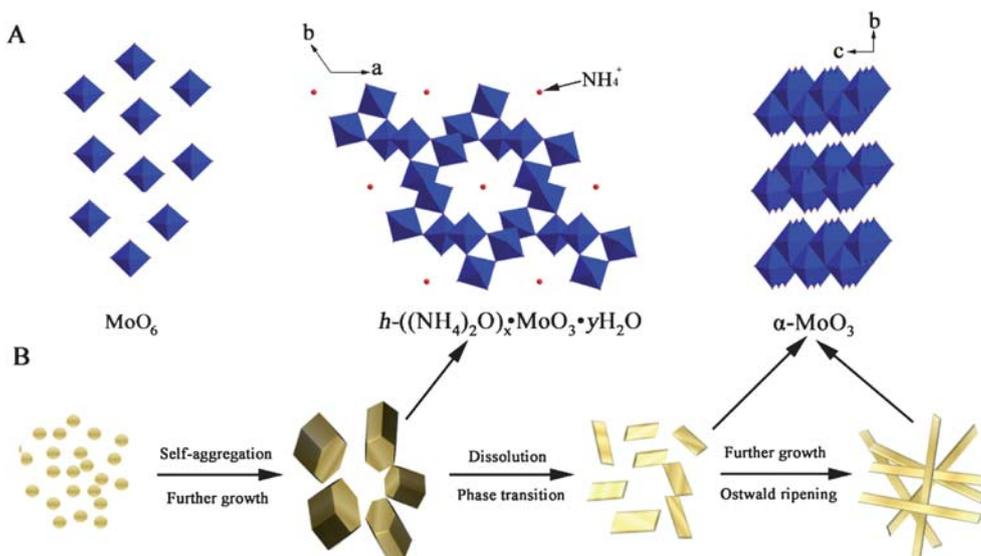
**Scheme 1** (A) Crystal structures of  $h\text{-}(\text{NH}_4)_2\text{O}_x \cdot \text{MoO}_3 \cdot y\text{H}_2\text{O}$  and  $\alpha\text{-MoO}_3$ ; (B) The probable growth mechanism of  $\alpha\text{-MoO}_3$  nanobelts
