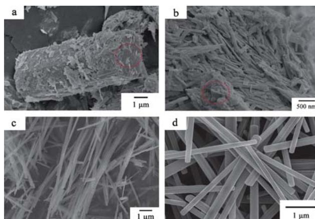
Fig. 9 SEM images of the products collected at different reaction time intervals in the presence of TX-10 (reaction temperature = 180 °C): (a) 5 min, (b) 0.5 h, (c) 5 h, (d) 20 h.
