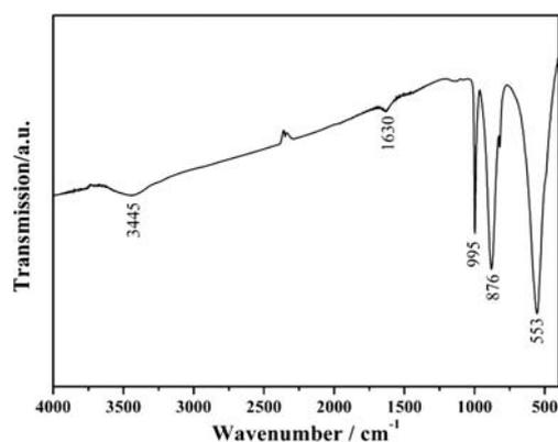
Fig. 6 FT-IR spectrum of the as-synthesized MoO<sub>3</sub> nanobelts.
