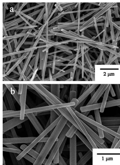
Fig. 2 Typical SEM images of the as-synthesized MoO<sub>3</sub> nanobelts: (a) low-magnification SEM image; (b) high-magnification SEM image.
