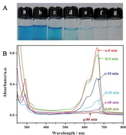
**Fig. 11** (A) Photo images and (B) absorption spectra of MB solution ( $10 \text{ mg L}^{-1}$ ,  $100 \text{ mL}$ ) in the presence of  $50 \text{ mg MoO}_3$  nanobelts at different time intervals.
