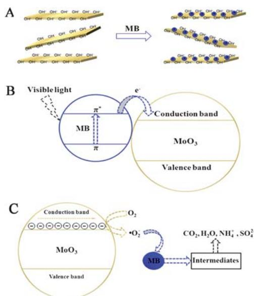
**Scheme 2** Possible mechanism for the photodegradation of MB under visible light. (A) MB is adsorbed at the surface of  $\alpha$ - $\text{MoO}_3$  nanobelts; (B) MB absorbs visible light to induce the  $\pi$ - $\pi^*$  transition, the excited-state electrons then readily inject into the d-orbital (CB) of  $\text{MoO}_3$ ; (C) the excited-state electrons react with adsorbed oxygen to yield superoxide radicals  $\cdot\text{O}_2^-$  and then MB is mineralized by the radicals.
