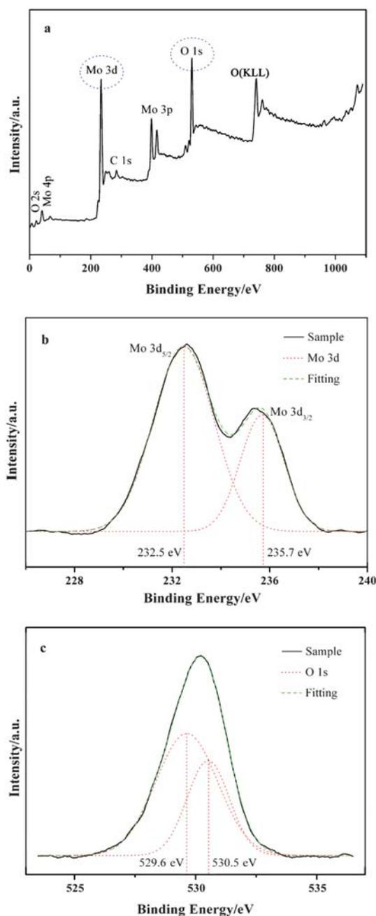
**Fig. 5** X-Ray photoelectron spectra of the as-synthesized MoO<sub>3</sub> nanobelts: (a) survey spectrum, (b) Mo 3d spectrum, (c) O 1s spectrum.
