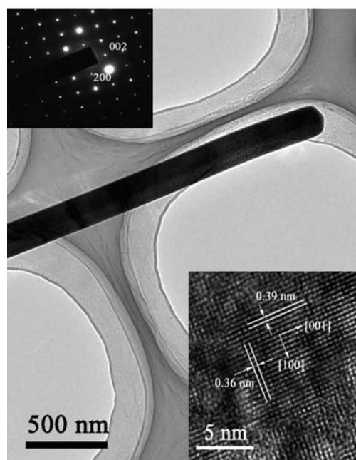
**Fig. 4** Typical TEM image of the as-synthesized MoO<sub>3</sub> nanobelts (inset: selected area electron diffraction (SAED) pattern and HRTEM image of an individual molybdenum oxide nanobelt).
