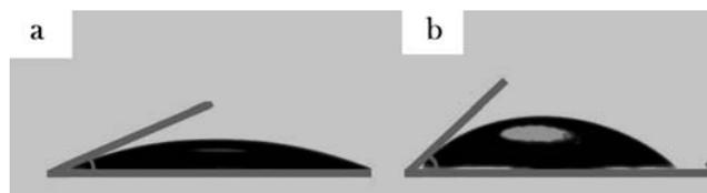
**Fig. 7** Contact angles of water on: (a) HOMGF/Ab-BSA/BMIm +  $\text{BF}_4^-$ -gel membrane and (b) HOMGF/Ab-BSA/BMIm +  $\text{PF}_6^-$ -gel membrane.
