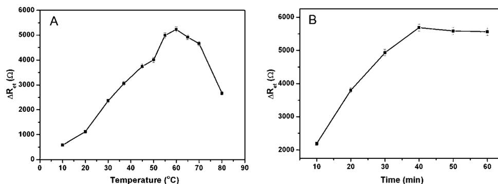
Fig. 3 Relationship of  $\Delta R_{et}$  with the incubation temperature (A) and incubation time (B) on the response of EIS.
