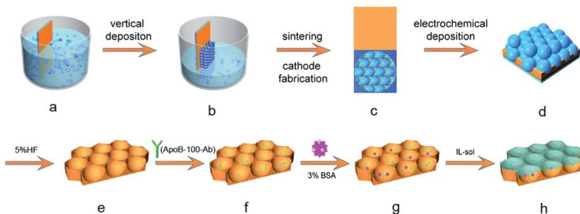
Scheme 1 Schematic Illustration of the Stepwise Immunosensor Fabrication
