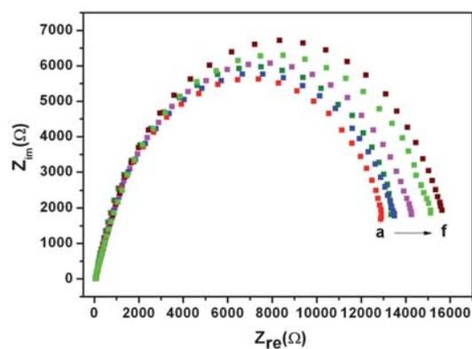
**Fig. 6** Faradaic impedance spectra corresponding to the control experiment with  $\text{BMIm}^+\text{PF}_6^-$  used as additive in IL-gel membrane, before and after incubating with different concentrations of ApoB-100 in PBS (20 mM, pH 7.0) solution containing 0.1 M KCl and 5 mM  $\text{Fe}(\text{CN})_6^{3-/4-}$ : (a) blank solution; curves b–f represent 0.005, 0.05, 0.5, 5.0 and 50.0 pg/mL ApoB-100, respectively.
