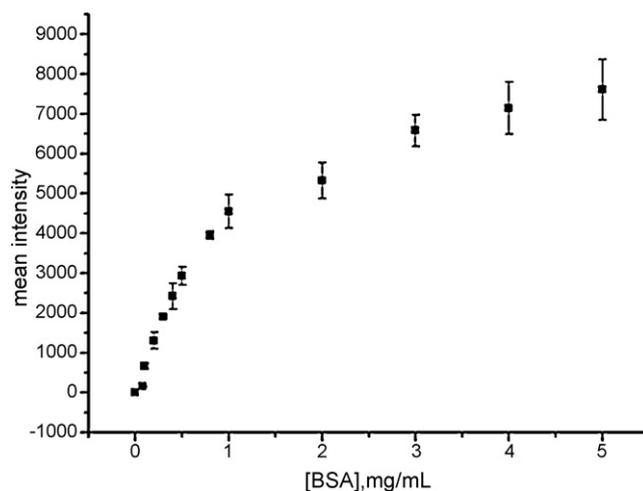
**Fig. 4.** Standard curve made from the data collected by a camera. Concentrations of BSA were between 0 and 5 mg/mL. Conditions: Olympus FE-210 digital camera, programmed auto exposure without flash light, the object distance is 30–40 cm. Darkness density was picked to analyze by image software Quantity One.
