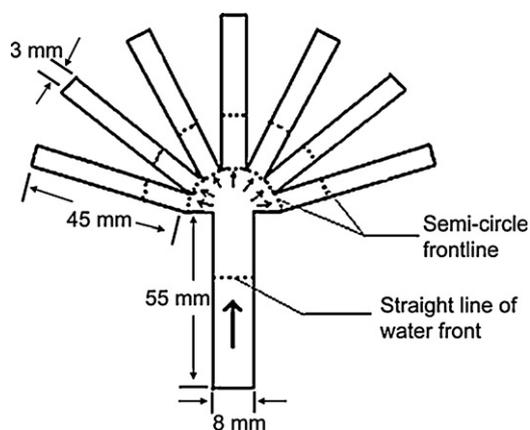
**Fig. 2.** Tree-shaped design ensures uniform conditions of each assay. The arrow shows the direction of water, indicating that the frontline of the water spreads from a straight line to a semi-circle when coming to a wider channel.
