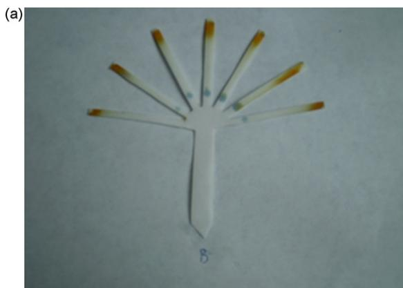
**Fig. 5.** (a) A tree-shaped paper device with a stem and seven branches after test. (b) A sample detection with a standard curve in the tree-shaped device. The red cross lies in the place of the sample with a mean intensity of 3475, reads 0.82 mg/mL in concentration, while the true value is 0.75 mg/mL. Conditions are the same as in Fig. 4.
