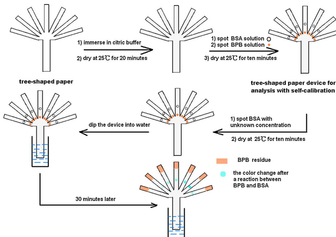
Fig. 1. Diagram of the procedure for tree-shaped device with self-calibration for detection.
