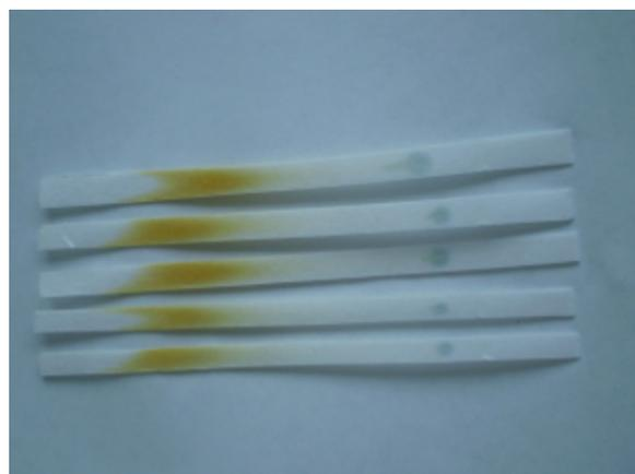
**Fig. 3.** Assays with BSA samples of the same concentration, but different volumes of 0.3  $\mu\text{L}$ , 0.5  $\mu\text{L}$ , 1.5  $\mu\text{L}$ , 2.0  $\mu\text{L}$  respectively (from the bottom to the top), indicate that volume of the sample solution does not affect the result in large extent.
