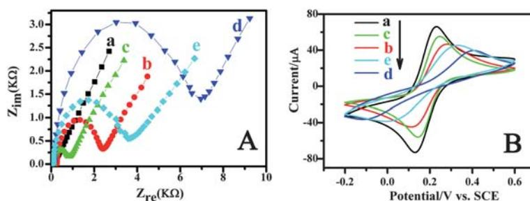
**Fig. 4** EIS (A) and CV (B) of the electrode at different stages in 0.1 M KCl + 2 mM  $[\text{Fe}(\text{CN})_6]^{3-/4-}$ . (a) bare Au electrode, (b) probe/Au electrode, (c) ATP/probe/Au electrode, (d) cDNA/ATP/probe/Au electrode, (e) QDs/cDNA/ATP/probe/Au electrode. The EIS frequency range:  $0.1\text{--}1.0 \times 10^5$  Hz. The CV scan rate was  $100 \text{ mV s}^{-1}$  and the ATP concentration  $18 \mu\text{M}$ .
