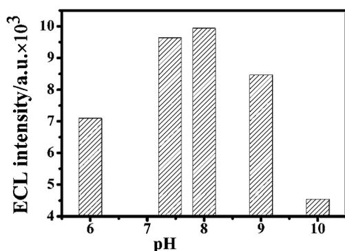
**Fig. 6** Effect of pH on the ECL response of the aptasensor. The electrolyte: PBS<sup>+</sup> solution containing 0.1 M K<sub>2</sub>S<sub>2</sub>O<sub>8</sub> and 0.1 M KCl with pH value range from 6.0, 7.4, 8.0, 9.0 to 10.0. The voltage of the photomultiplier tube was 600 V and the scan rate 100 mV s<sup>-1</sup>.
