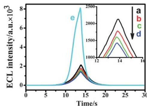
**Fig. 5** ECL intensity of different modified electrodes. (a) bare Au electrode, (b) probe/Au electrode, (c) ATP/probe/Au electrode, (d) cDNA/ATP/probe/Au electrode, (e) QDs/cDNA/ATP/probe/Au electrode. The inset is the amplification of curve (a), (b), (c) and (d). The electrolyte: 5 mL pH 7.4 PBS<sup>+</sup> solution containing 0.1 M  $\text{K}_2\text{S}_2\text{O}_8$  and 0.1 M KCl. The voltage of the photomultiplier tube was 600 V and the scan rate  $100 \text{ mV s}^{-1}$ .
